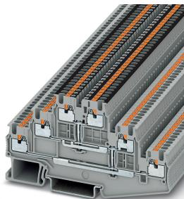
Multi-level terminal block, With equipotential bonder, nom. voltage: 500 V, nominal current: 15 A, connection method: Push-in connection, 1 level, Rated cross section: 1.5 mm<sup>2</sup>, cross section: 0.14 mm<sup>2</sup> - 1.5 mm<sup>2</sup>, mounting type: NS 35/7,5, NS 35/15, color: gray
