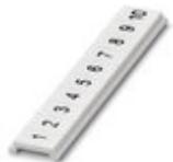
Zack Marker strip, flat, Strip, white, labeled, printed horizontally: consecutive numbers 1 ... 10, 11 ... 20, etc. up to 91 ... 100, mounting type: snap into flat marker groove, for terminal block width: 3.5 mm, lettering field size: 5.15 x 3.5 mm, Number of individual labels: 10
